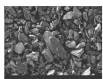
Figure 4. Micrograph of wet applied granilho
